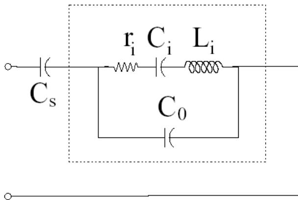
$$-\frac{i * X_0 * (r_1 + i * X_1 - i * X_{c1})}{r_1 - i * X_0 + i * X_1 - i * X_{c1}} - i * X_s$$
