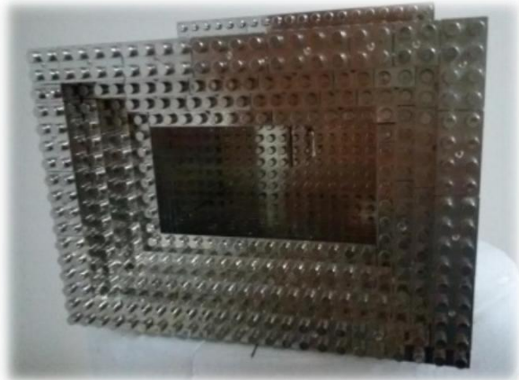
80 mm X 52 mm (A X B) Antenna Gain: 9.2 dBi Azimuth HPBW: 55°
