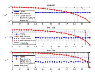
Fig. 3. Comparison between the analytical expression obtained for  $\rho$  and the actual crossing point OSTBC and beamforming curves.
