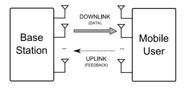
Fig. 1. Point-to-point MIMO system.
