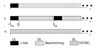
Fig. 4. Proposed scheme: I. No motion: feedback once then use beamforming; II. Small motion: increase rate of feedback, and use beamforming; III. Fast motion: no feedback and OSTBC.
