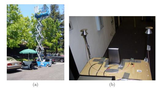
Figure 1: (a) Base station antennas at the transmitter lifted to 10m, (b) Receive arrays used for the O2I moving measurements
