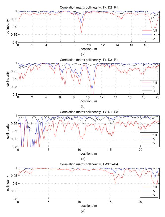
Figure 5: Collinearity of correlation matrices for four different combinations of transmitter positions and routes.
