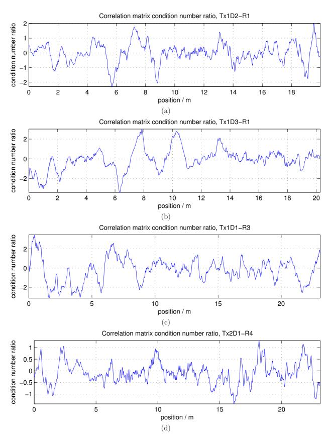
Figure 6: Condition number ratio of the full correlation matrices for four different combinations of transmitter positions and routes.
