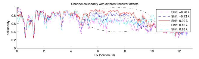
Figure 7: Collinearity of channel matrices of measurement Tx1D1-R3, when the two measured routes show a small position offset.
