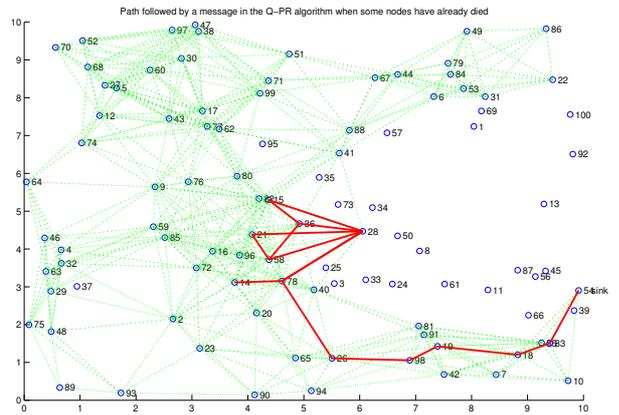
**Fig. 2:** Illustration of network topology and routing path between node  $N_{14}$  and the sink node (node  $N_{54}$ ). Discontinuous links show neighborhood relationships. Dead nodes have no discontinuous connection lines.
