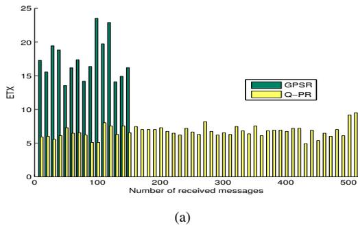
**Fig. 3:** Temporal evolution of ETX for a single simulation concerning to groups of 10 messages received by destination for the GPSR and Q-PR algorithms.
