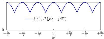
Sampled noise z[n] is white because the ambiguity function of  $f(t) = f_b(t)$  is a triangle with support between -T anx T, which sampled at symbol rate is a delta function.
