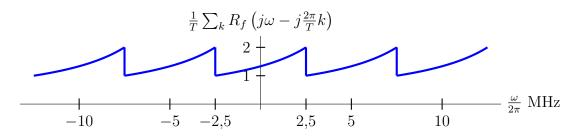
Exercise 1.16 (Solution) a) Joint transmitter-receiver response, in this case, is equal to the ambiguity function of the transmitter filter
