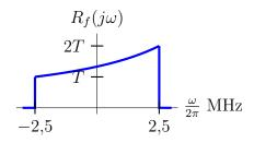
The addition of replicas of this response shifted multiples of  $\frac{2\pi}{T}$  rad/s is shown below
