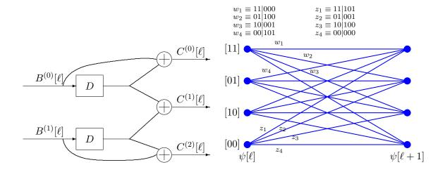
b) Generator matrix and trellis diagram for the second encoder
