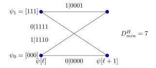
The concatenated code has better performance than both individual codes, because its minimum distances is much higher, allowing to correct up to 3 error in every block of 8 encoded bits.
