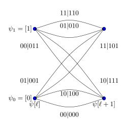
b) Trellis diagram is also shown in the previous figure (above). Minimum distance is
