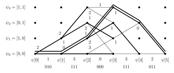
and table includes the accumulated metric for each state, with boldface highlighting the metric of the survival path. Finally, decoded bits are provided.
